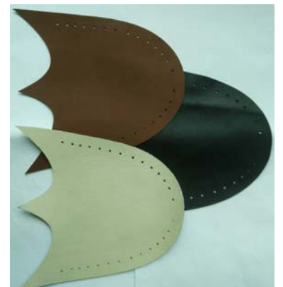
Cutting sample on leather & PU
