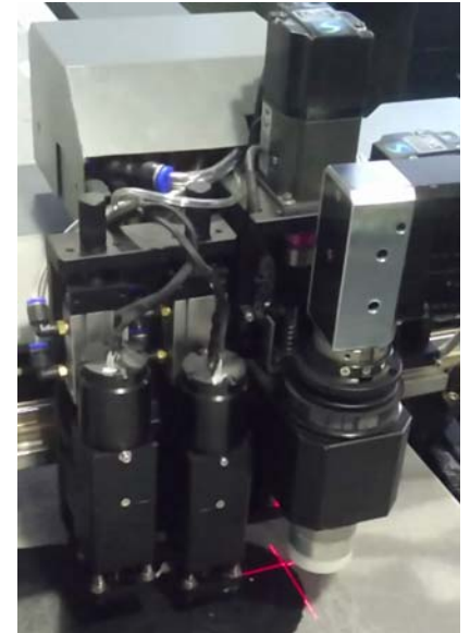
Oscillating Tool with 2 hole punching tools
